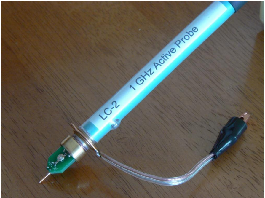
Fig. 1: Probe body with 10:1 Dc-coupled tip and ground lead attached.
