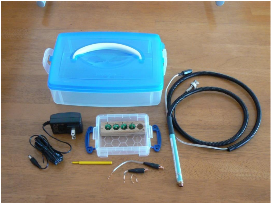
Fig. 2: The probe kit, as supplied. A slip-on aluminum shield (not shown) is also included. The power converter is shown with a North American mains connector. Connectors for other regions are available.
