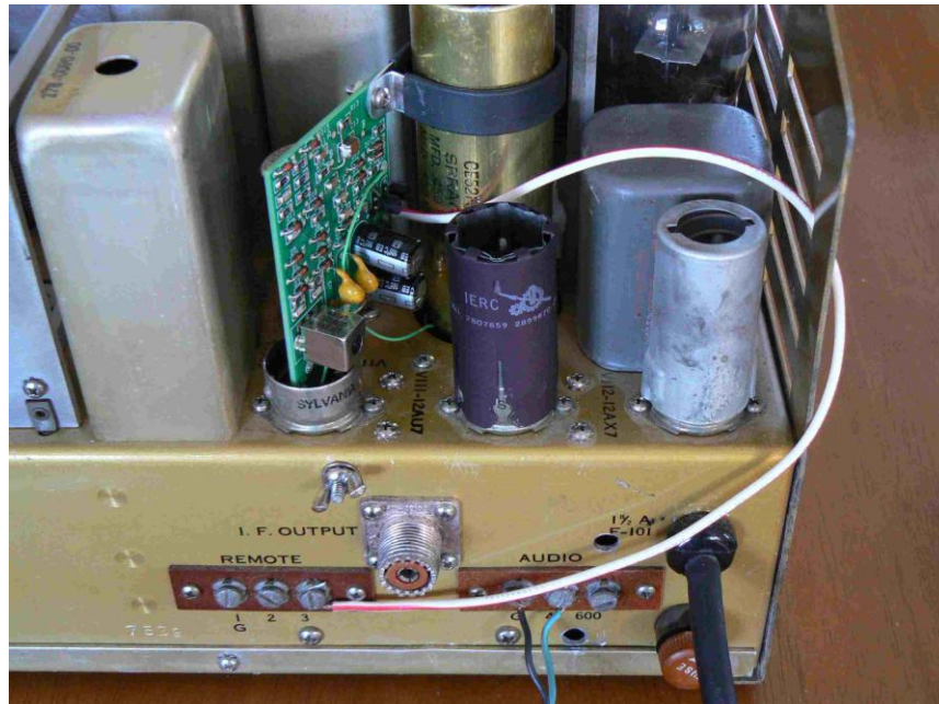
Fig. 2 – As installed in the receiver. The white wire supplies 12 volts to the muting relay. You can also leave it out, or route it below the chassis and solder to the terminal inside the receiver.
