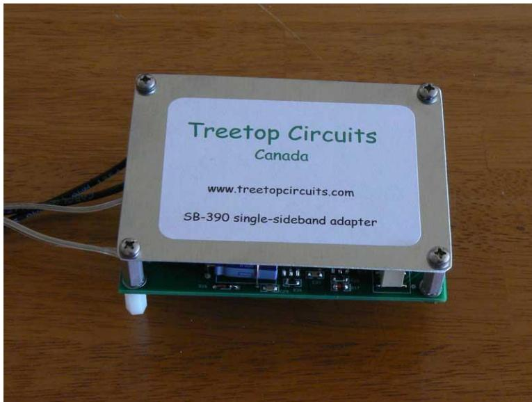
*Fig. 4B: Standoffs and cover on top side*
