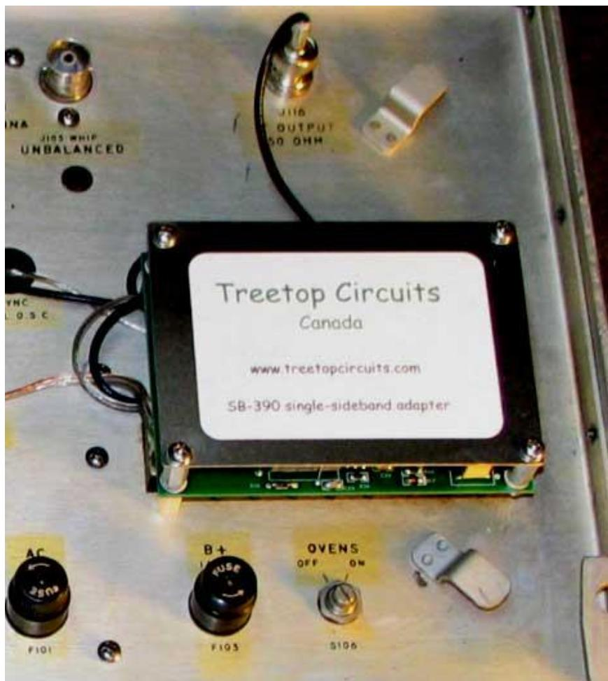
Fig. 2: An SB-390 installed on an R-390A
