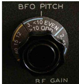
*Fig. 6 – This setting actually produces the same result as Fig. 5. You'd use it for Band 13, which is >10 megacycles and odd-numbered.*
