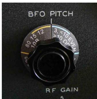
*Fig. 3 – The BFO PITCH knob with stickers.*
