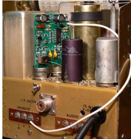
*Fig. 2 – As installed in the receiver. The white wire (optional, to be supplied by owner) supplies 12 volts to the muting relay. You can also leave it out, or route it below the chassis and solder to the terminal inside the receiver.*
